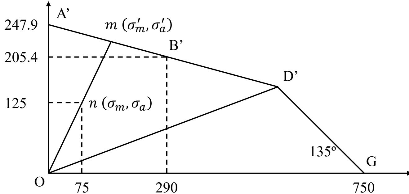
Then analyze the position of the working stress state point. Since  $\sigma_0 = 580\text{MPa}$ ,  $\sigma_{-1} = 350\text{MPa}$ , then
